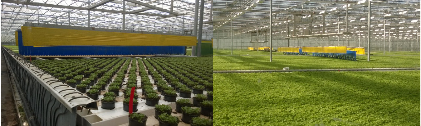
Figure 3. Irrigation booms with hanging plastic are programmed to brush plants throughout the day to control plant height. Photo courtesy of Paul Fisher.
