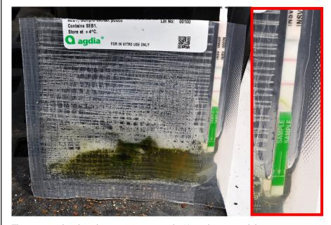
This is a test kit that shows a positive result. Note the two pink lines on the test strip.
