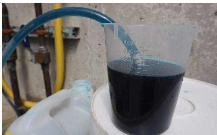
Figure 3. The injector siphon inside the graduated cylinder with a concentrated fertilizer stock solution.
