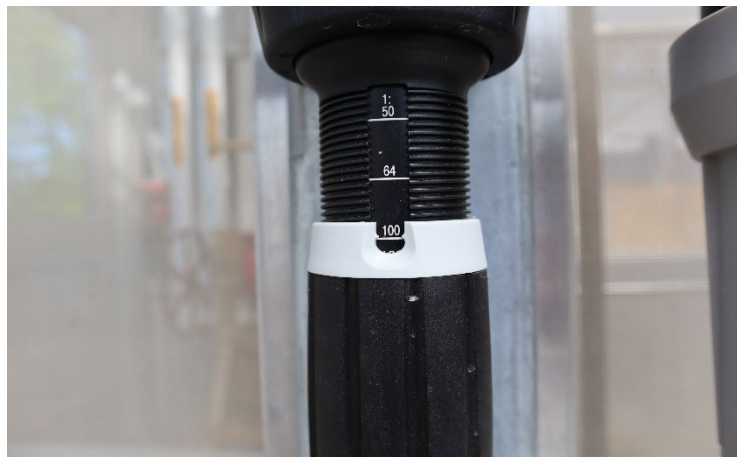
Figure 2. Setup of the injector at a 1:100 dilution ratio.
