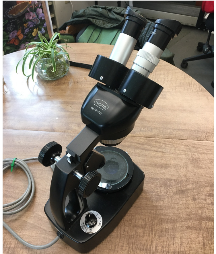
Older Wolfe stereoscope with ring zoom (around objective lens) and both incident and transmitted light sources built in. Note the individual adjustment on one eyepiece
