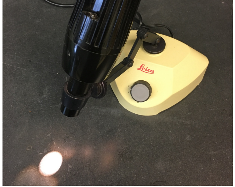
Older Leica light source for stereoscope. Light level is adjustable. We used these years ago until fiber optic and LED units were available.
