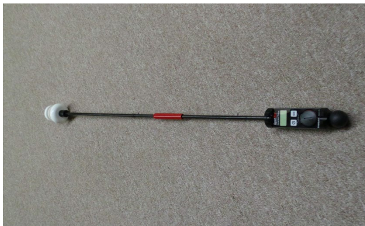
Figure 2: Thermal Inversion Tester for use in determining if temperature inversions exist prior to spraying. (Photo - Tom Ford Penn State Extension)
