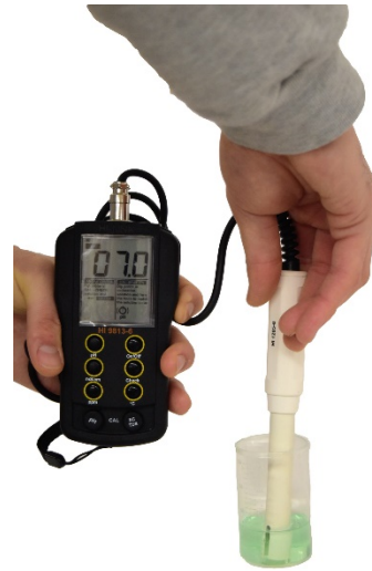
Figure 10. While waiting 30 minutes, calibrate the pH/EC meter. Photo by: W. Garrett Owen.
