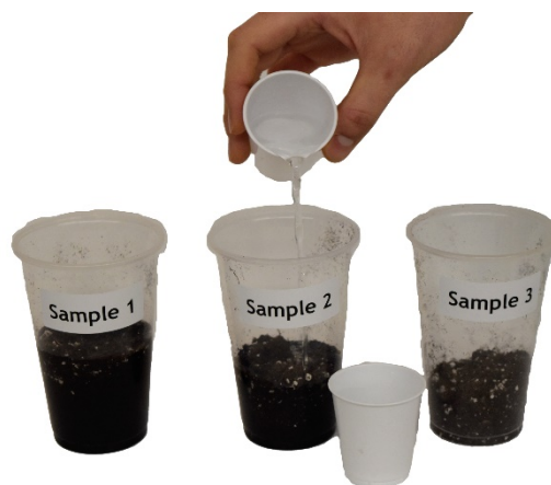
Figure 8. Add 6 ounces of distilled water (2 parts by volume) to the substrate subsample. Photo by: W. Garrett Owen.
