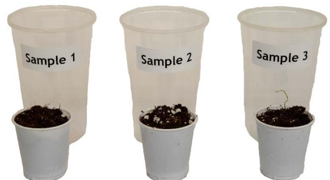
Figure 6A. Three ounce cups are used to extract three representative subsamples from the moistened substrate sample. Photo by: W. Garrett Owen.
