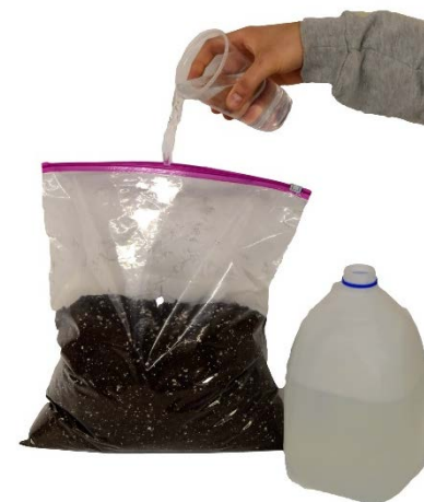
Figure 2. Moistening the substrate sample by adding distilled water. Photo by: W. Garrett Owen.
